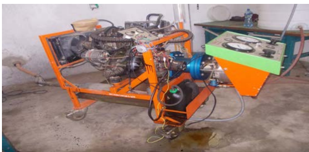
Figure 1: Experimental setup of Hydraulic dynamometer on diesel engine Test rig
